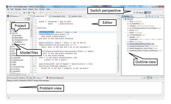
Figure 3.1: The Overture Perspective
