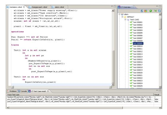
Figure 3.14: Using Combinatorial Testing for the Alarm VDM-SL model
