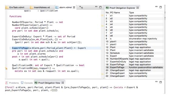
Figure 3.16: The Proof Obligation view for the Alarm VDM-SL model
