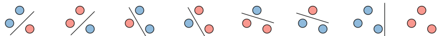
Figure 2.2: In two dimensions, we can shatter any three non-collinear points. VC dimension of a linear classifier in 2D equals 3.
