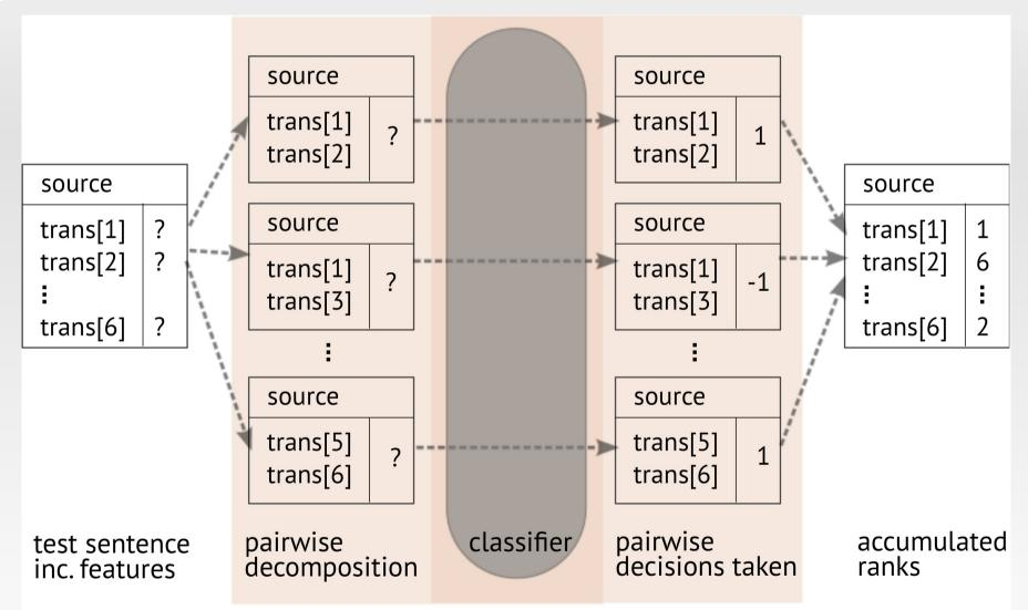
The process of Machine Ranking, performed through pairwise comparisons for 6 system outputs
