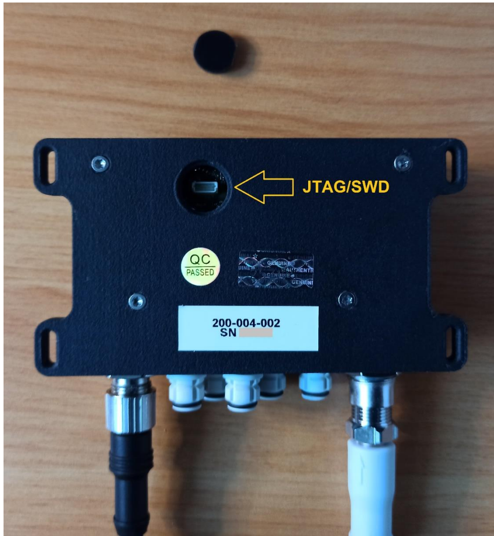
JTAG/SWD connector under a blind grommet
