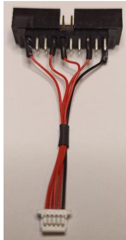
Wiring a JTAG/SWD Adapter to the ST-LINK/V2 debugger
