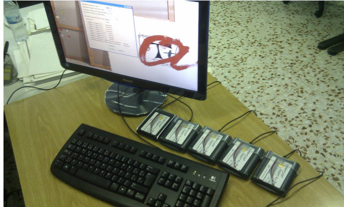
Figure 4.1: This picture shows the PC with the main application in execution and the set of SC readers connected.
